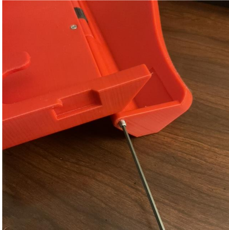
Install M4x6mm Set Screws on both sides of the hinge.
