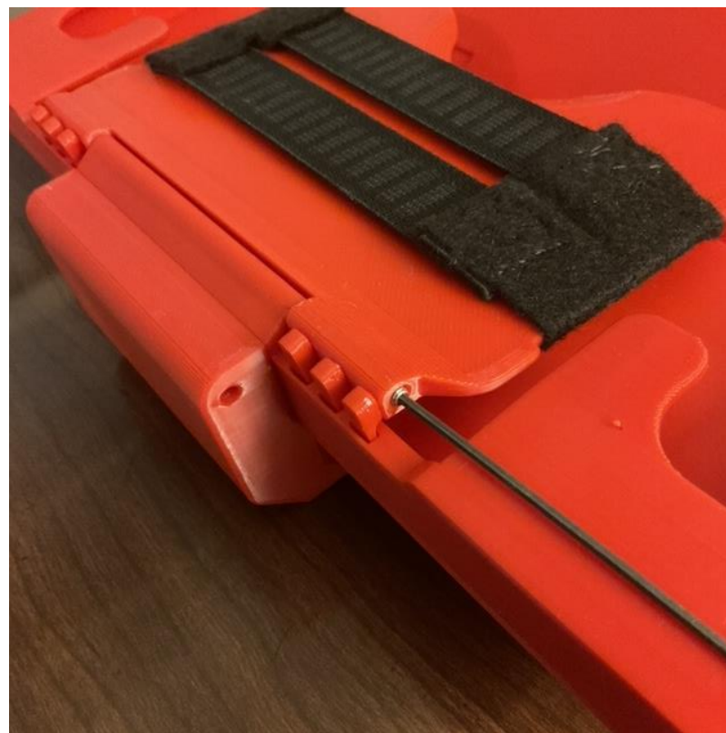
Install the M3x6mm Set Screw
