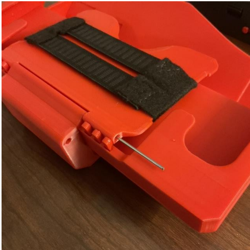
Install the 95mm lg. 1.5mm Dia. Pin
