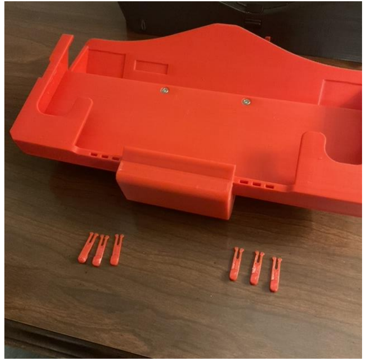
These are the springs used for the bistable hinge used in the screen protector. They slide into the slots at the base of the print.
