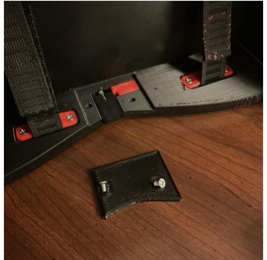
Install the latch and latch stop. Slide the latch cover plate down then screw into place.
